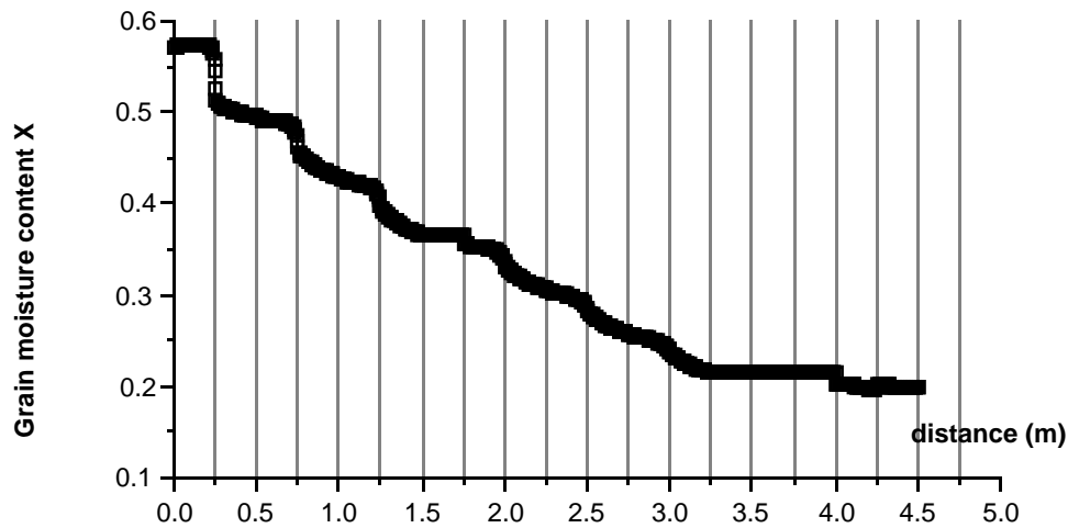
Figure 4.9: Test 2 / 1987 - simulated evolution of the grain moisture content X in the course of its descent (abscissa oriented from the top to the bottom of the dryer).
