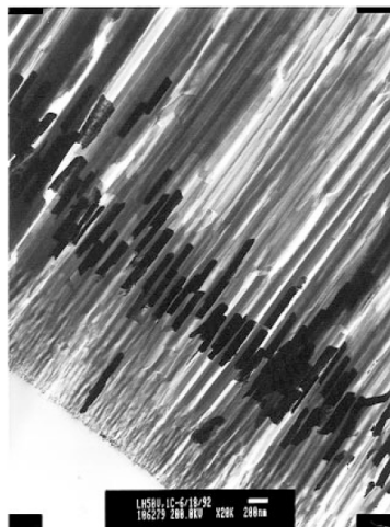
Figure 5: Transmission electron micrograph of an alumina template membrane showing 70 nm diameter Au nanowires within the pores. ?
