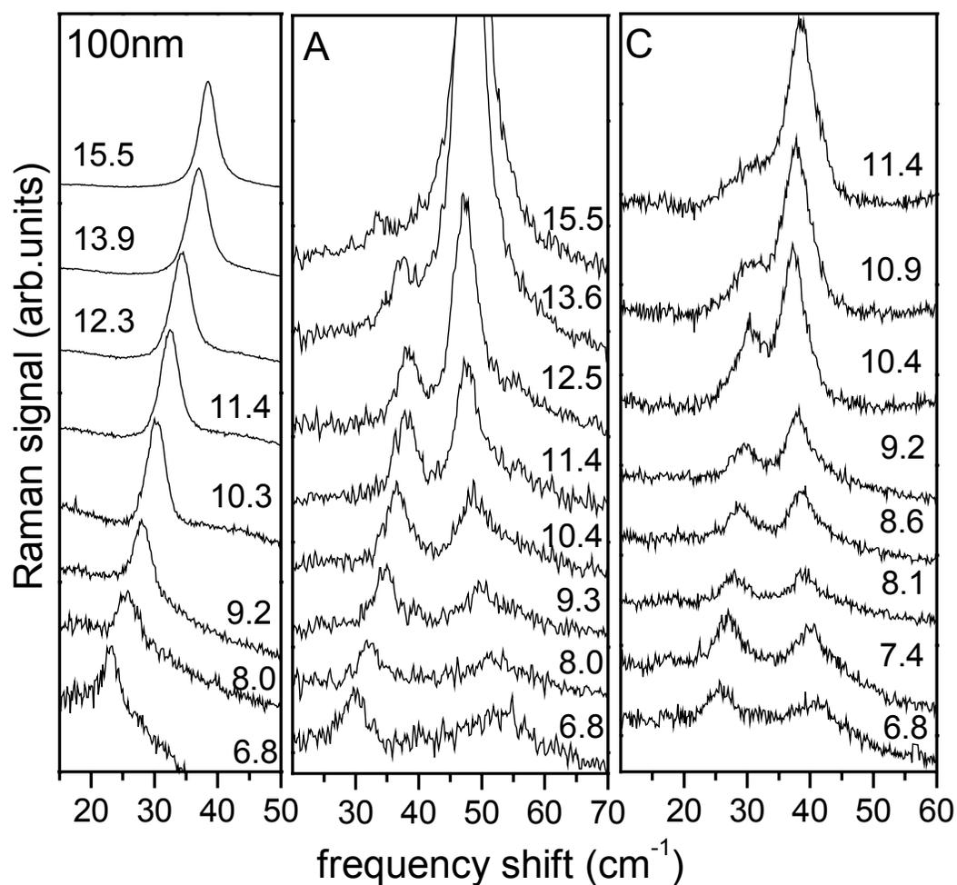
**Fig.2** Raman spectra obtained in parallel polarization on sample A, sample C and a 100nm wide unmodulated wire, for different values of the wavevector along the wire axis. This parameter is given in  $\mu\text{m}^{-1}$  for each spectrum in the figure.
