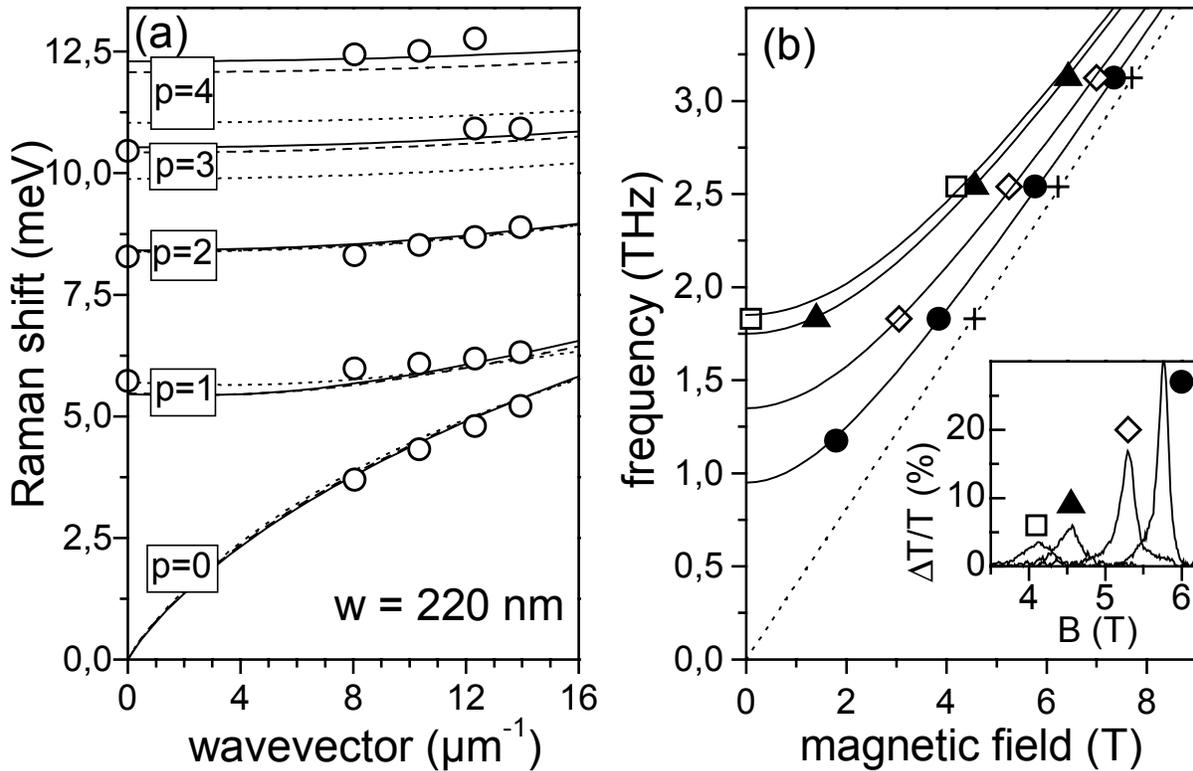
**Fig.1a:** Plasmon dispersions determined by RS experiments (open circles) compared with calculated dispersions using  $n=4$  (dotted lines),  $n=10$  (dashed lines) and  $n=\infty$  (solid lines).  $p$  labels the different confined plasmons.
