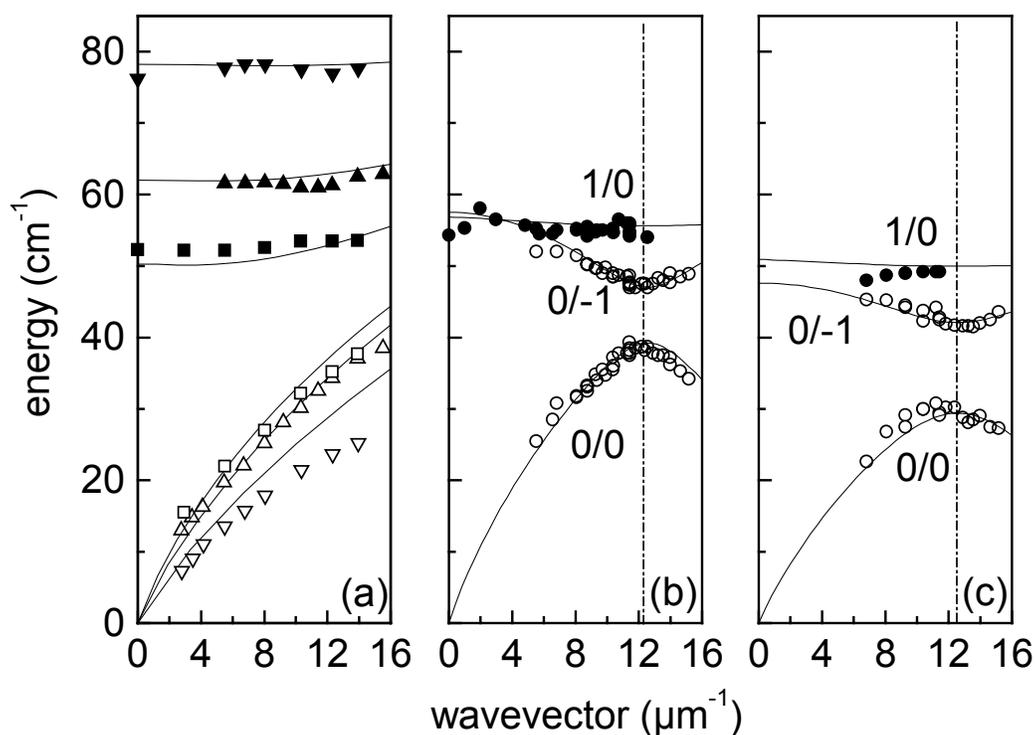
**Fig.3** Comparison between experimental and theoretical plasmon dispersions along the wire axis for mode 0 (open symbols) and mode 1 (closed symbols) in a) three unmodulated wires with different widths: 60 (down triangles), 100 (up triangles) and 180nm (squares) and in two different modulated wires: b) sample A and c) sample B.
