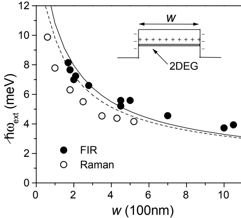
**Fig.3:** FIR resonance position at  $B=0$  and  $p=1$  RS peak energy at  $q=0$  for the various investigated samples (symbols). The dashed and solid lines are the dependence  $\omega_{\text{ext}}(w)$  calculated using a trapped electron density of  $2.5 \times 10^6 \text{ cm}^{-1}$  and  $6.5 \times 10^6 \text{ cm}^{-1}$  respectively. The wire model used in the calculations is shown in the inset.
