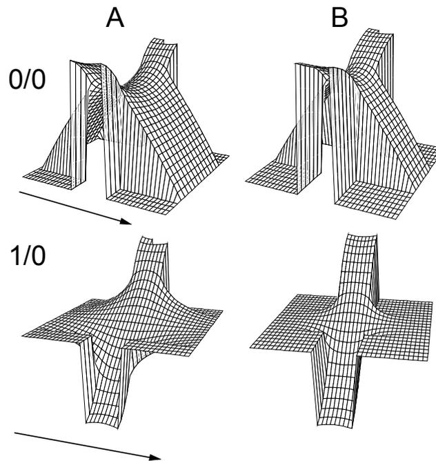
**Fig.4** Fluctuations of the electrostatic potential associated with the folded plasmon mode  $0/0$  and the confined one  $1/0$ , calculated at zone edge for sample A and B respectively. The arrows indicate the wire axis.
