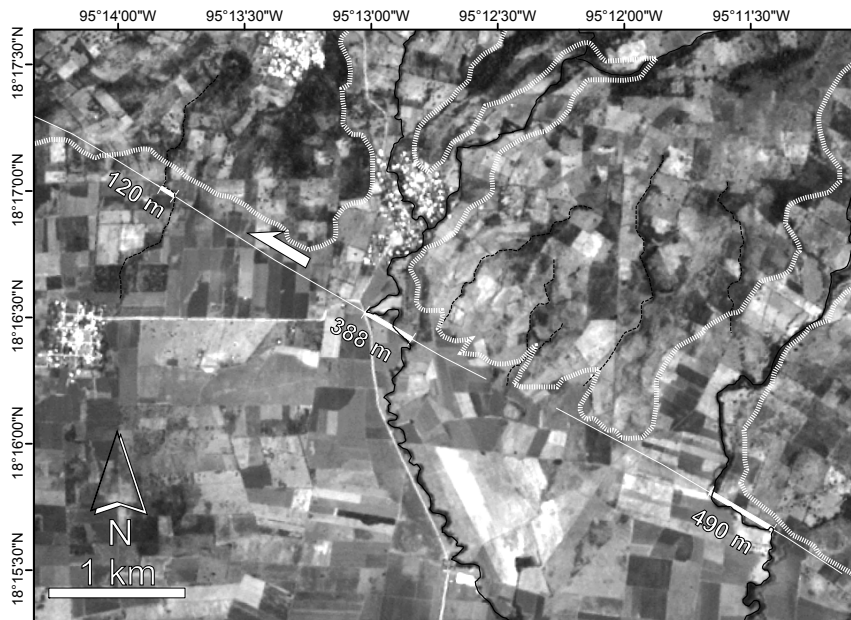
FIG. II.7 – SPOT satellite image of an area located in the southwestern part of the Los Tuxtlas Volcanic Field (location on fig. II-6). A discrete fault trace is evidenced here by systematic left-lateral river offsets and by the sharp termination of the volcanic plateau (white dashed lines).
