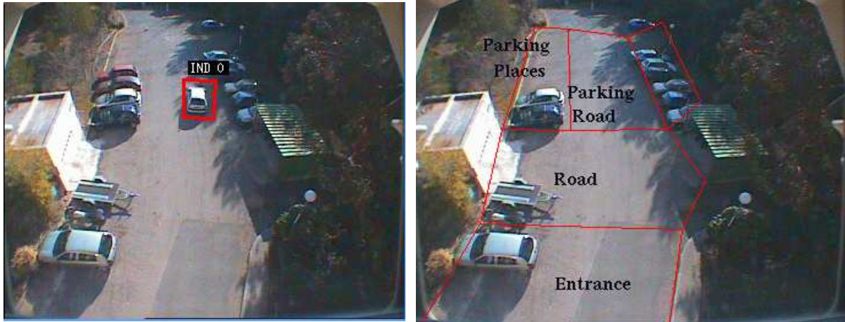
Figure 9.11: (a) Visualization of the event 'vehicle on the parking road'. (b) Manually defined zones in the scene.
