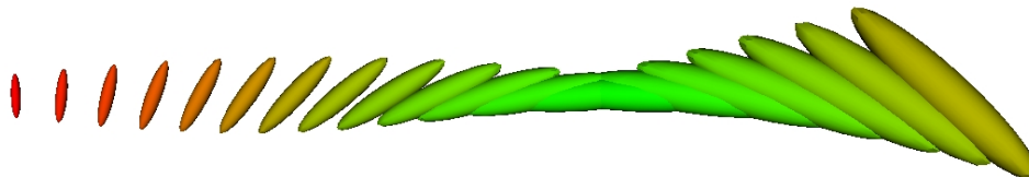
Figure 3.1: Independent interpolation of tensor eigenvectors and eigenvalues. A re-orientation step is necessary to prevent this behavior to occur: the interpolated tensors seem not to take the most direct path between the two extremities.
