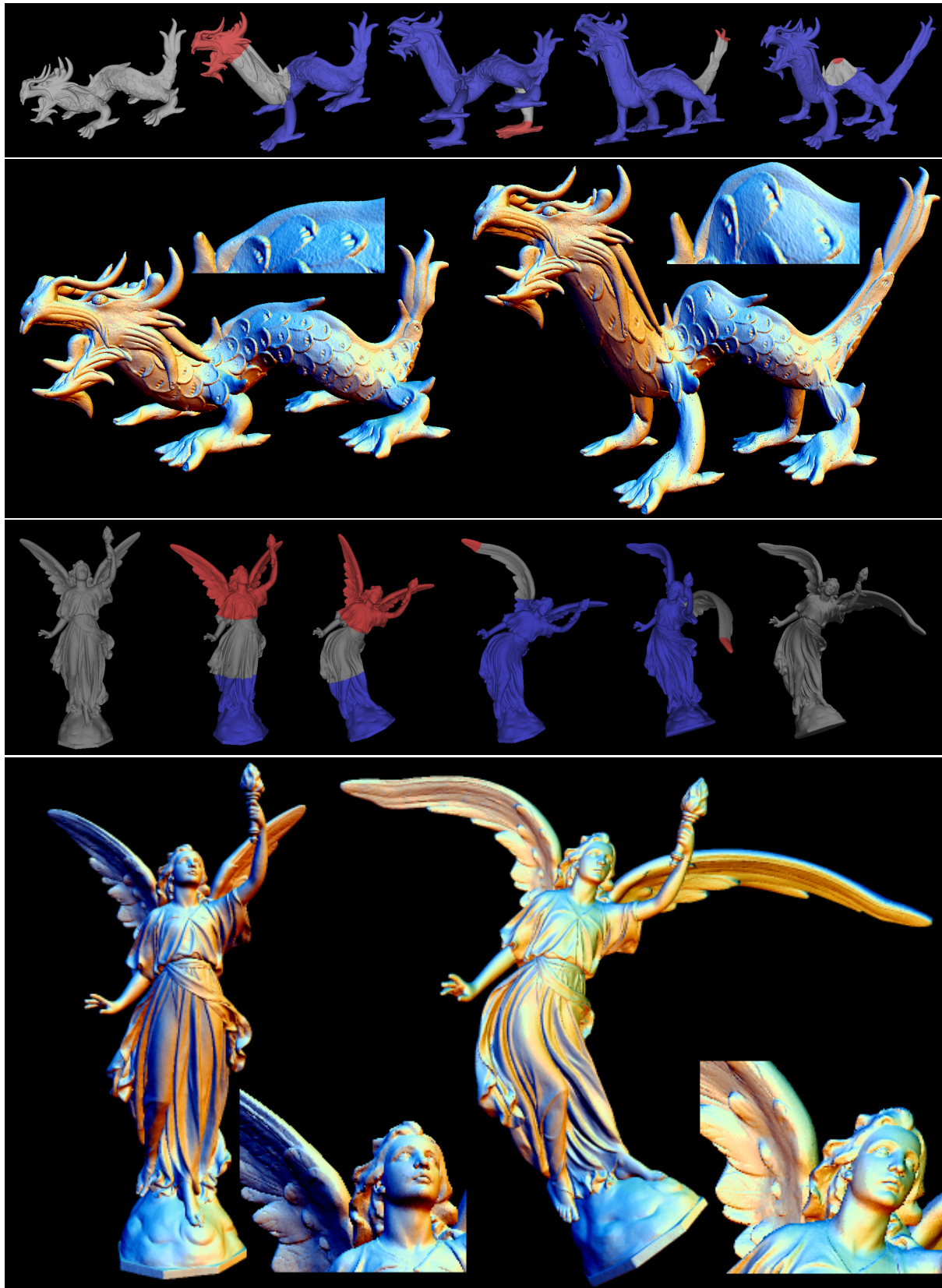
Figure 4.14: Interactive freeform deformation of very large models. Top: XYZRGB Dragon (7M triangles) - 160k samples for interactive deformation. Bottom: Lucy (28M polygons) - 300k samples for interactive deformation. Interaction snapshots are displayed in grey, red and blue. Each full session with adaptive simplification, interactive editing and deformation transfer took less than 5 minutes.
