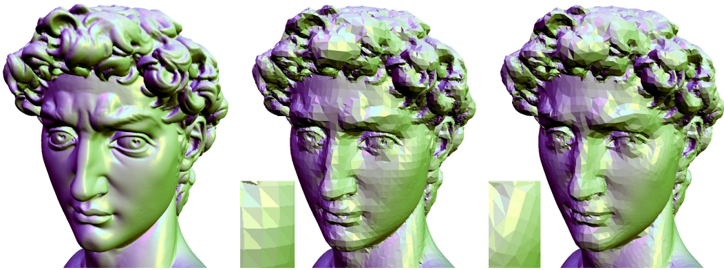
Figure 3.4: Hierarchical mesh simplification with L^2 error bounded at 2.10^{-3} . Left: Original object (7M triangles). Middle: Octree simplification (1.75 sec. - 62856 triangles). Right: VS-Tree simplification (1.20 sec. - 52024 triangles).
