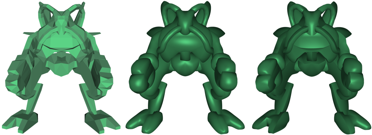
Figure 7.8: Left: Coarse mesh (1246 triangles on CPU). Middle: Adaptive interpolated smoothing by Curved PN Triangles (1.1M generated triangles on GPU). Right: Sharp features, tension and bias control with Scalar Tagged PN Triangles (similar number of generated triangles on GPU).
