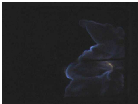
Fig. 3.3: View of the flame from underneath taken through the window in the floor of the compartment: line burner, large soffit, 0.36 \text{ }^{\circ}/_s fuel flow rate ( \dot{H} = 17 \text{ kW} ), unrestricted vent
