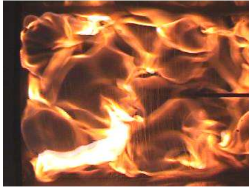
Fig. 3.7: View of the flame from underneath taken through the window in the floor of the compartment: line burner, large soffit, 0.71 \frac{\text{g}}{\text{s}} fuel flow rate ( \dot{H} = 33 \text{ kW} ), unrestricted vent
