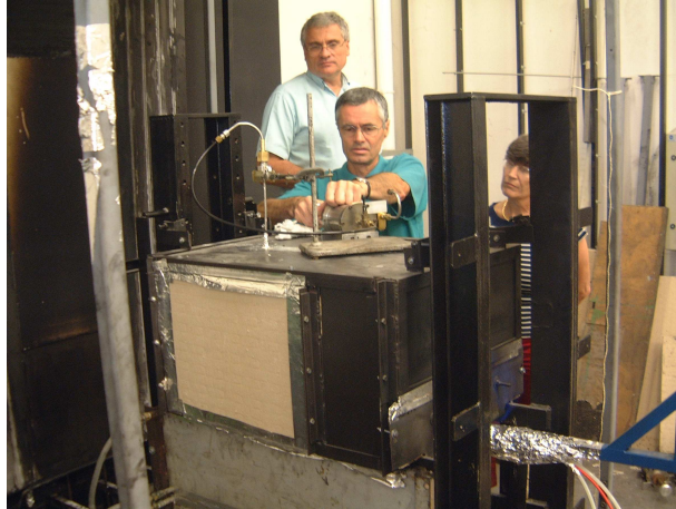
Fig. 2.13: A sample being taken for analysis the with the gas chromatograph
