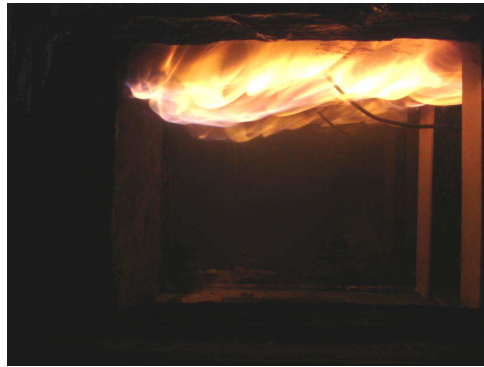
Fig. 3.29: View from the side of the flame for a fuel flow rate of 0.71 s/s [ \dot{H} = 33 kW] and a vent width of 0.2 m = 0.5 W
