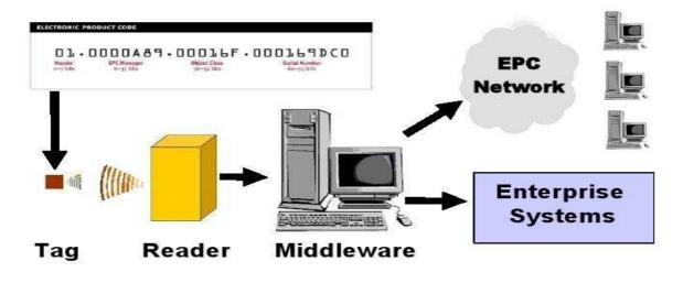
Figure 1.1: RFID System Components, source: Confino and Elmore [4]
