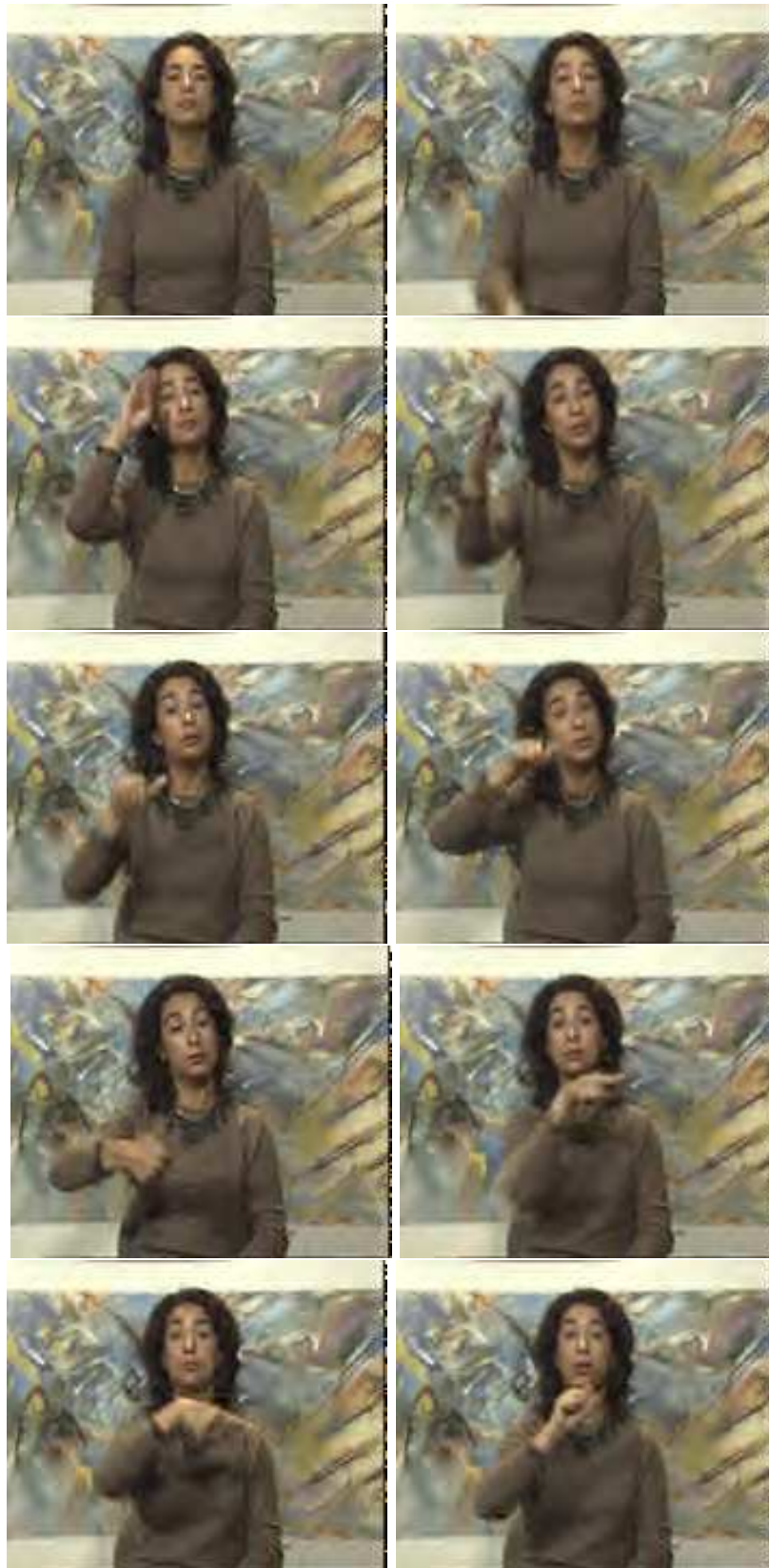
Figure 4.28: QCIF silent color video compressed at 200 kbits/s (30 frames/s). Transmission over UMTS Pedestrian channel at 0.001 ber. Using the proposed MDC.
