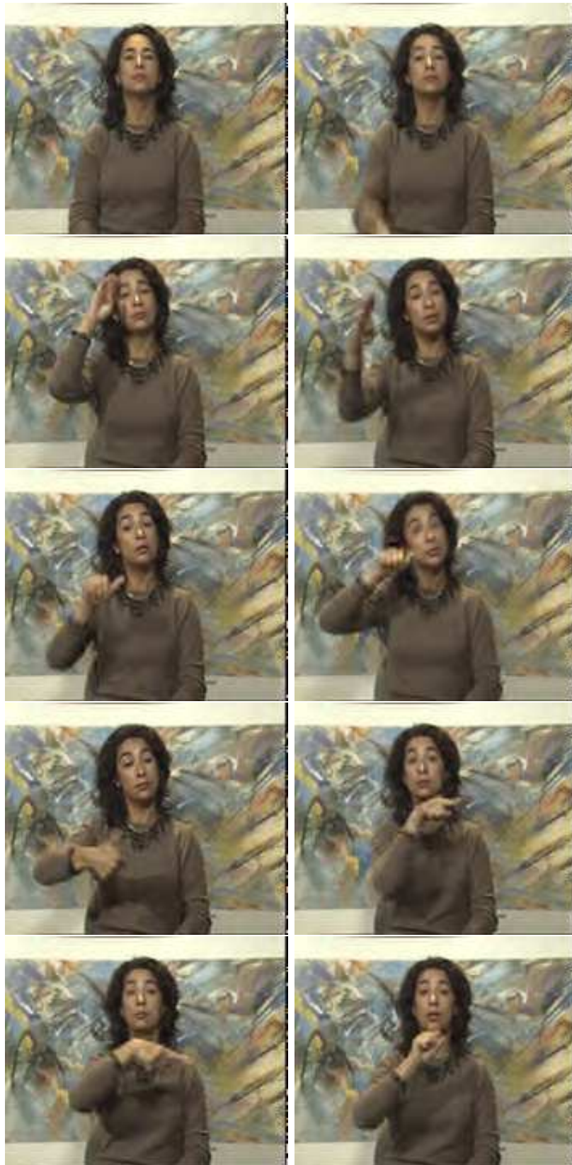
Figure 4.26: QCIF silent color video compressed at 200 kbits/s (30 frames/s). Transmission over UMTS Pedestrian channel at 0.001 ber. Using SDC without channel coding.
