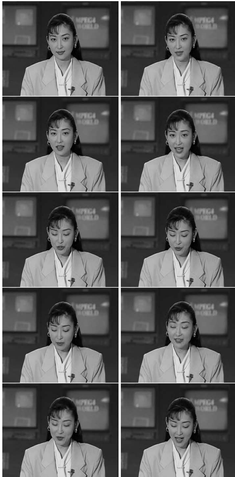
Figure 4.16: CIF akyio video compressed to 300 kbits/s (30 frames/s). Transmission over Gaussian channel at 0.001 ber. Using the proposed MDC.
