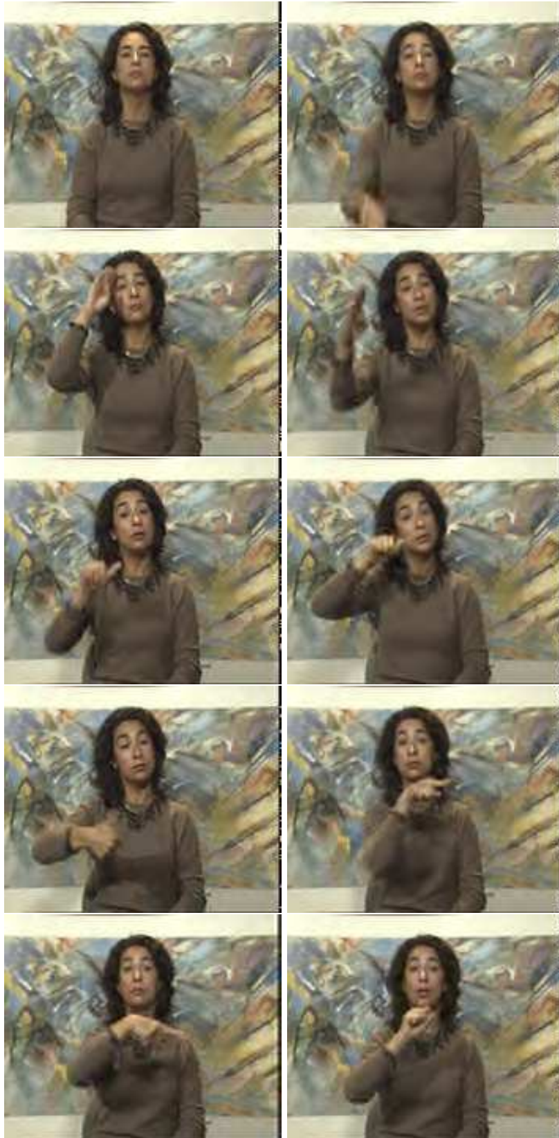
Figure 4.14: QCIF silent color video compressed to 200 kbits/s (30 frames/s). Transmission over Gaussian channel at 0.001 ber. Using the proposed MDC.
