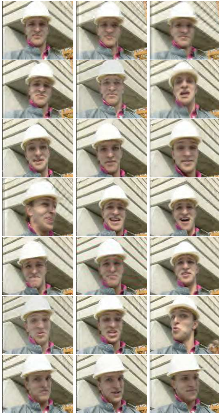
Figure 4.33: QCIF Foreman color video compressed at 200 Kbps (30 frames/s). Transmission over an Internet simulator suffering from 5 % packet loss. Using the proposed MDC. Y-PSNR: 26.76 dB; U-PSNR: 38.82 dB; V-PSNR: 40.52 dB.
