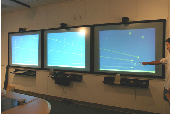
Figure 4: Moving an object using the drag-and-pop technique on the iWall wall-size display.
