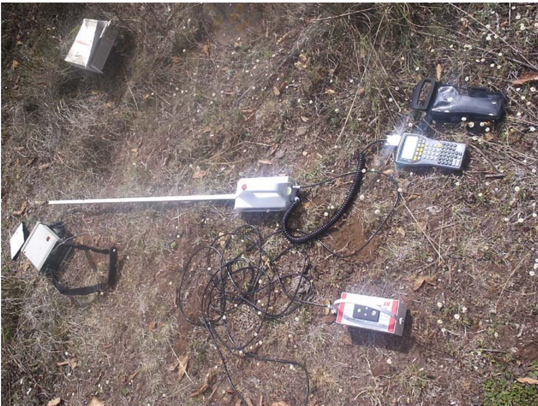
Photograph A.10: Spectroradiometer and ceptometer on soil of oak forest plot, Cuitzeo.
