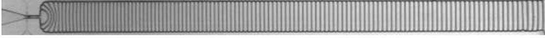
Figure 4.24: Compressible foam flow at high flow rate, Q_l = 43 \mu\text{l}/\text{min} and P_g = 35 \text{ kPa} , L = 16 \text{ mm} .
