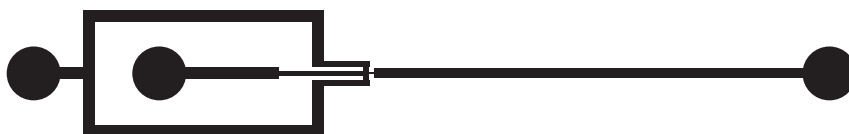
Figure A.5: Ultraflat channel. h = 8 \mu\text{m} , w_{or} = 75 \mu\text{m} , l_{or} = 200 \mu\text{m} , w = 400 \mu\text{m} , L = 20 \text{ mm} .
