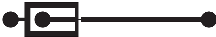
Figure A.1: Classic geometry. h = 250 \mu\text{m} , w_{or} = 100 \mu\text{m} , l_{or} = 400 \mu\text{m} , w = 700 \mu\text{m} , L = 17 \text{ mm} .
