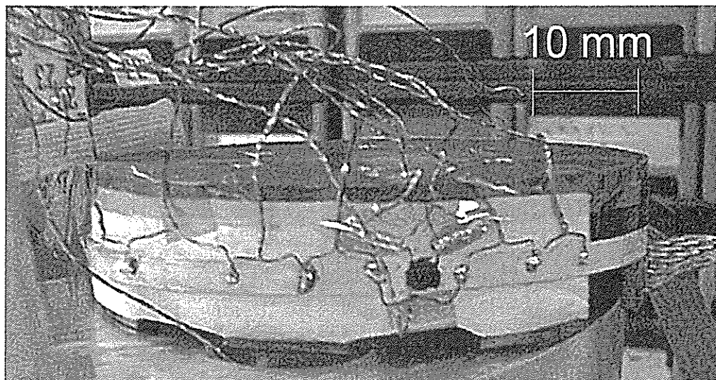
Figure VI.19: OFHC copper sample holder for quasi-adiabatic measurements, on which is mounted a Bi-2223 tape.
