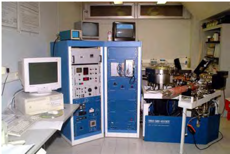
Figure 3: Photo du ToF-SIMS PHI Evans TRIFT I au CEMEF.
