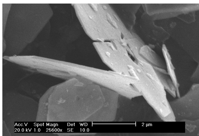
Figure II.6 – MEB. Alumine lamellaire.
