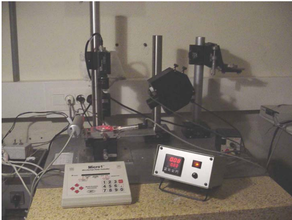
Figure 4-9: Photograph of the complete blister system
