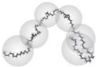
Figure 2.3: Representation of a polymer molecule and a corresponding coarse grained model
