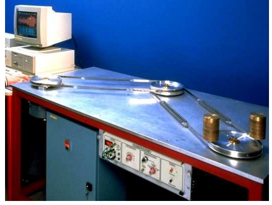
Fig. 2. View of the flexible transmission
