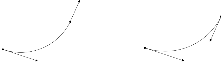
Fig. 6.1. Left: Usual Langevin dynamics; in this case, it is very unlikely to re-obtain the initial configuration starting from the final one. Right: Momentum reversal after integration time \Delta t ; in this case, the dynamics is reversible.
