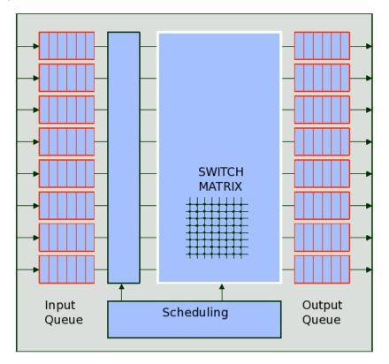
Figure 4.13: Generic NoC router microarchitecture
