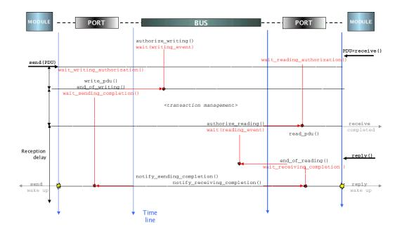
Figure 5.8: Send/Receive protocol example
