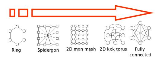
Figure 4.4: Example of networks topologies
