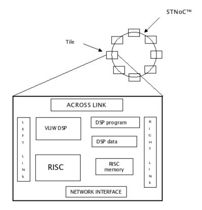
Figure 8.2: STNoC<sup>TM</sup> in a multi-tile parallel architecture
