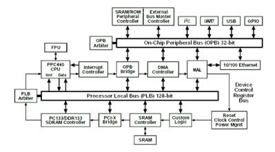
Figure 3.5: CoreConnect Based System-on-a-chip
