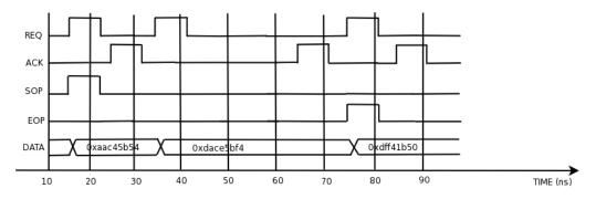
Figure 5.11: Standard router link protocol handshake
