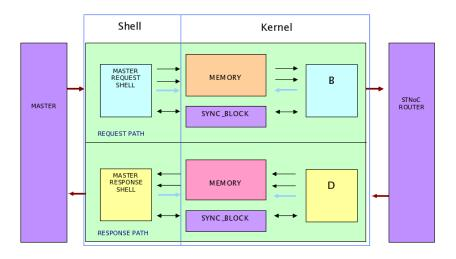
Figure 5.15: Mock-up of a NI microarchitecture
