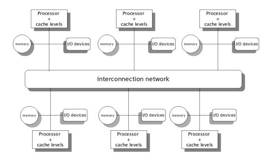
Figure 4.11: NUMA multiprocessors architecture
