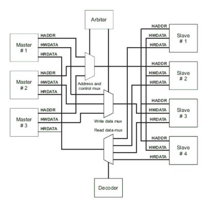
Figure 3.3: AHB bus microarchitecture
