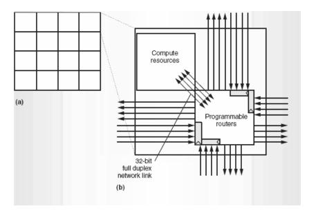
Figure 3.13: RAW on-chip interconnect a) RAW 16 tiles architecture b) Each tile has computational resources and four networks, each with eight pointto-point 32-bit buses
