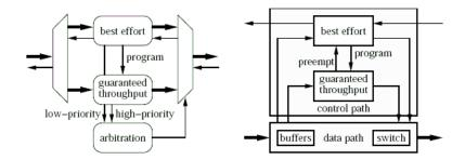
Figure 3.12: Overview of an Æthereal router
