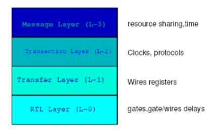
Figure 5.5: TLM stack of communication layers
