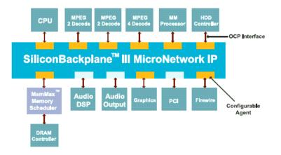
Figure 3.8: Example of Silicon backplane III integration in a multimedia SoC
