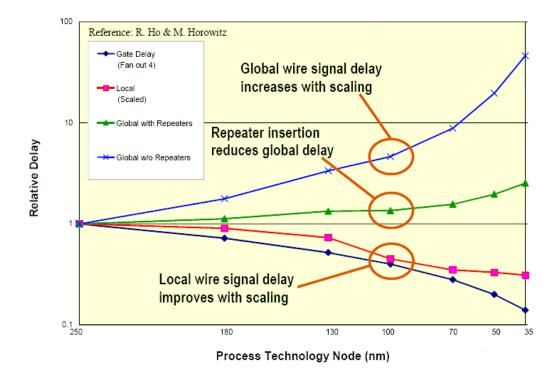
Figure 3.1: Local vs. Global wires delay
