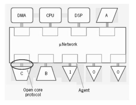
Figure 3.9: IP blocks integration in a network architecture
