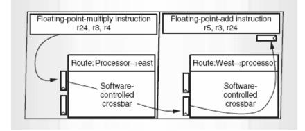
Figure 3.14: Two RAW tiles communicating over a static network
