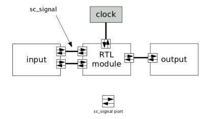
Figure 5.2: SystemC sample RTL model
