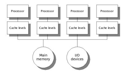
Figure 4.10: UMA multiprocessors architecture
