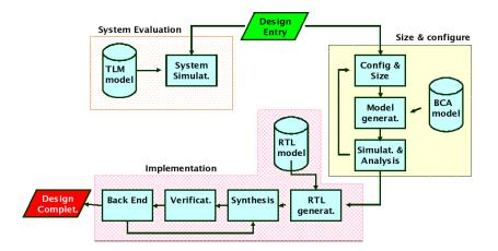
Figure 6.2: STBus genkit design flow
