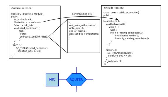
Figure 5.9: Example of protocol implementation through MsgBox functions
