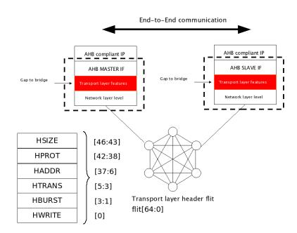
Figure 4.9: AHB end-to-end connection  $\$
