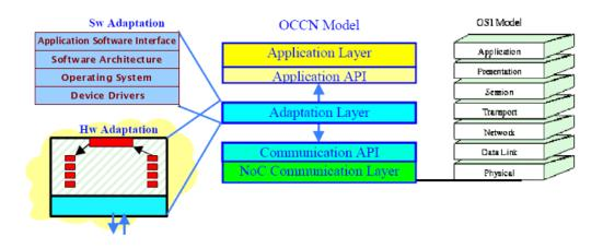
Figure 5.6: OSI like OCCN layering model
