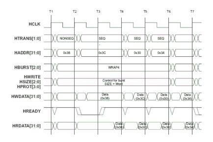
Figure 4.8: AHB wrap4 burst transaction
