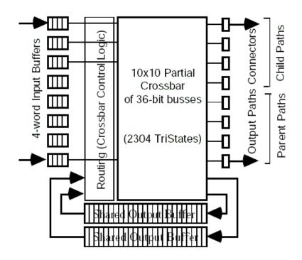
Figure 3.11: SPIN router macrocell microarchitecture
