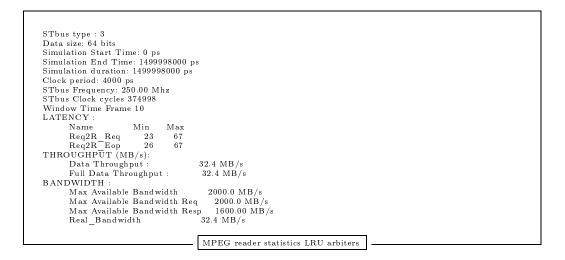
In the embedded snapshot the most interesting fields of Sysprobe concerning NoC benchmarking are reported. Some values are computed statically (e.g. max available bandwidth) whilst others are sampled dynamically. The snapshot above reports outcomes of an MPEG read process initiator whose bandwidth is around 30 Mbytes/sec. As it is an STBus initiator, latency is measured as delay between assertion of request and response request, in number of cycles.
