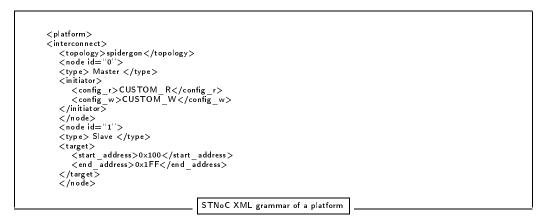
The given platform is instantiated as a Spidergon topology, with two nodes configured as a master and a slave. It is possible to declare the slave address space and initiator configuration files. This "STNoC<sup>TM</sup> explorer" turned out to be very useful to explore different NoC architectures and some results will be reported and highlighted in chapter 7.
