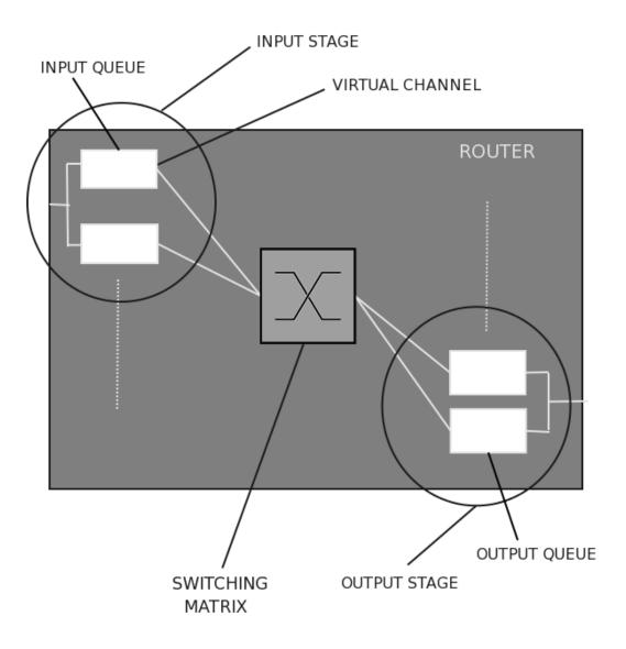
Figure 5.10: Standard router sketched micro-architecture
