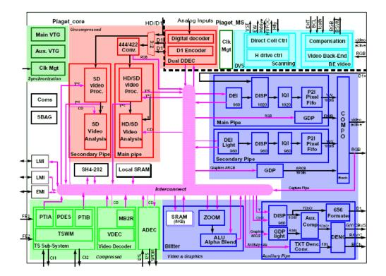
Figure 6.1: An example of a STMicrolectronics SoC
