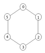
Figure 4.5: 6-nodes ring topology to demonstrate adaptive routing
