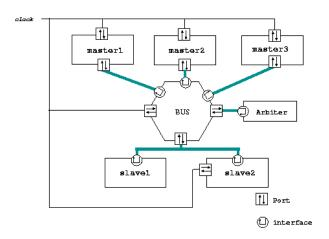
Figure 5.4: SystemC Simple Bus TLM structure
