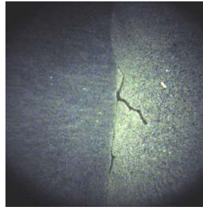
Figure A.II.6. Macro-cracks in the WJP91 welded component at the fusion line
