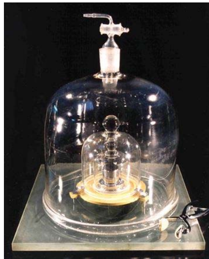
Figure I.1. : Prototype international du kilogramme \mathfrak{K} [photo BIPM]
