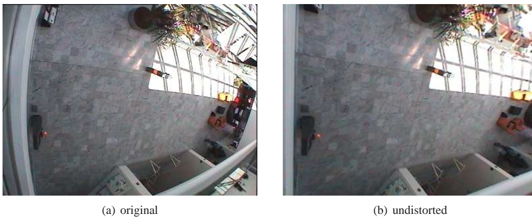
Figure 7.3: Distortion correction on hall images. The effect is noticeable in the curvature of the left white line which appears in both images. Remark that a part of the original image is lost in the process
