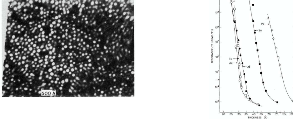
Figure 5.1: Left : Image of a granular film composed of Al grains on amorphous Ge background. The typical size of the grains is \sim 120 , [Shapira83]. Right : The granular structure of thin samples can be revealed studying the behaviour of the resistance in function of the thickness of the film. The nearly exponential behaviour shown in the figure can be justified only by a strongly non-uniform morphology typical of granular metals.
