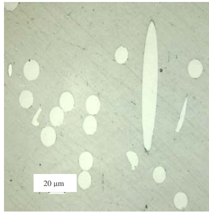
Figure 3. 25 – Bonne adhérence fibre-matrice
