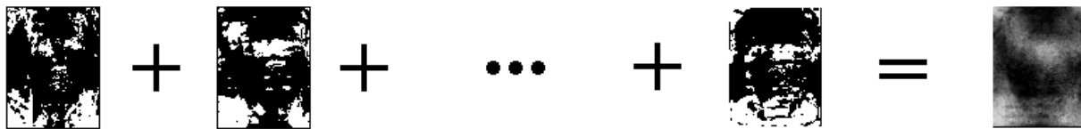
Figure 7.3: Example of salient facial regions detected on single images and their combination to a saliency map of a near frontal head pose. Dark pixel values represent non salient facial regions and light pixel values represent salient facial regions
