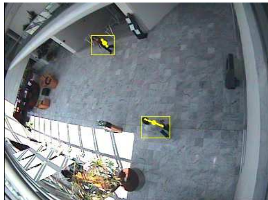
Figure 8.1: Image of a tracking sequence. The bounding boxes represent the regions of interest of tracked persons. The line represents the most significant ridge. The position and the orientation of the region interest is computed using the first and second moments of the difference image
