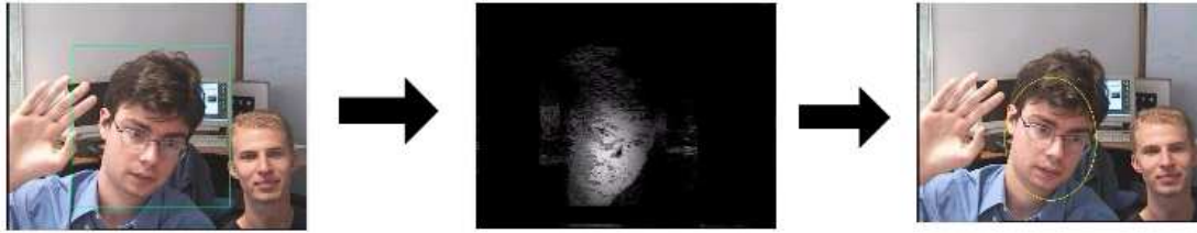
Figure 4.5: From left to right: ROI of a face in the image, Computation of the probability map multiplied by the Gaussian Window, Ellipse delimiting the face region in the image.
