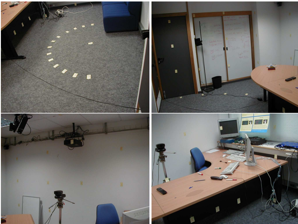
Figure A.4: Images from the FAME Platform of the PRIMA Team in INRIA Rhone-Alpes with the camera and the markers used for image acquisition
