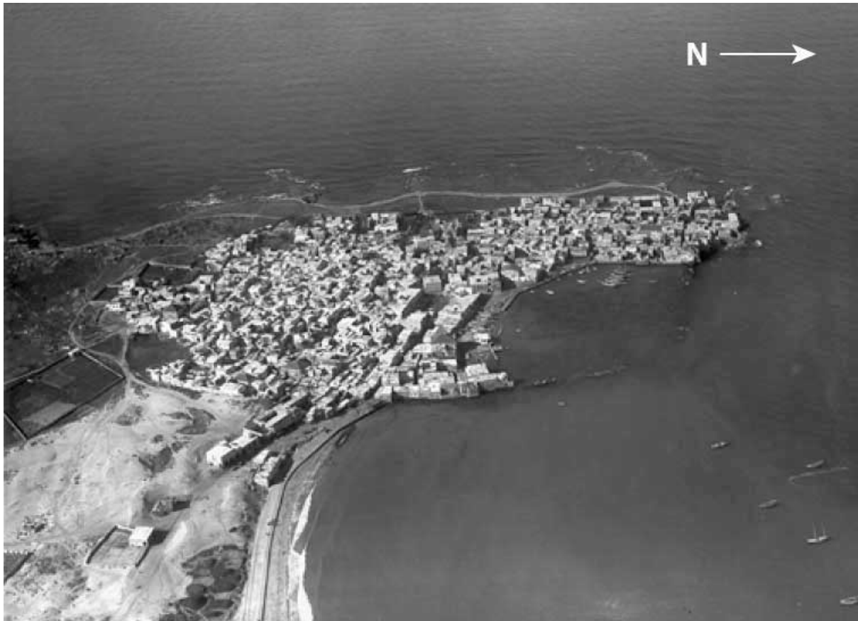
Figure 3.4: Oblique aerial view of Tyre's northern harbour around 1934, taken from the east (photograph: Poidebard archives at the Université Saint Joseph). The two medieval jetties are clearly visible in the picture. The ancient Iron Age/Roman breakwater is not manifest, but trends west-east from the eastern tip of the island.
