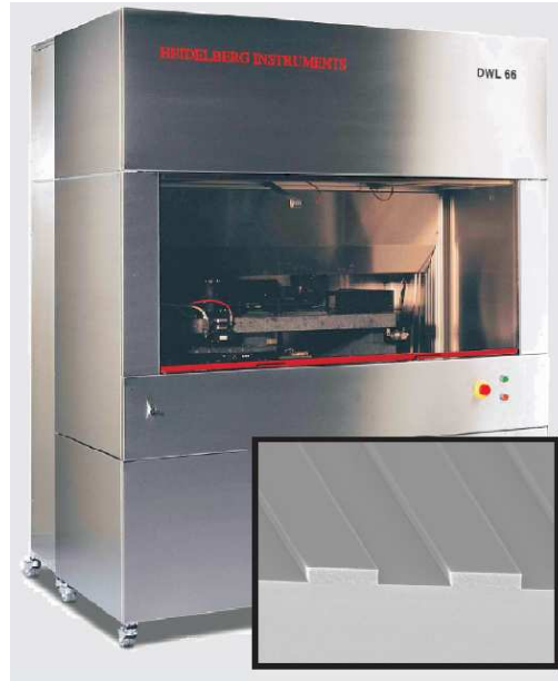
Figure 9.9: Direct writing laser 66 (DWL66) from Heidelberg instrument available at CSL.
