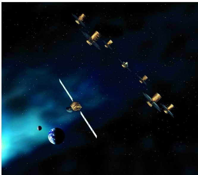
Figure 1.16: Darwin space interferometer’s six telescopes (original configuration), central view combining spacecraft, and communication satellite at L2. ©ESA.
