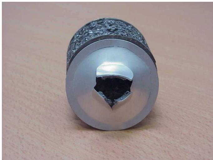
FIGURE 3.20: *Post-perforation de la plaque secondaire.*
