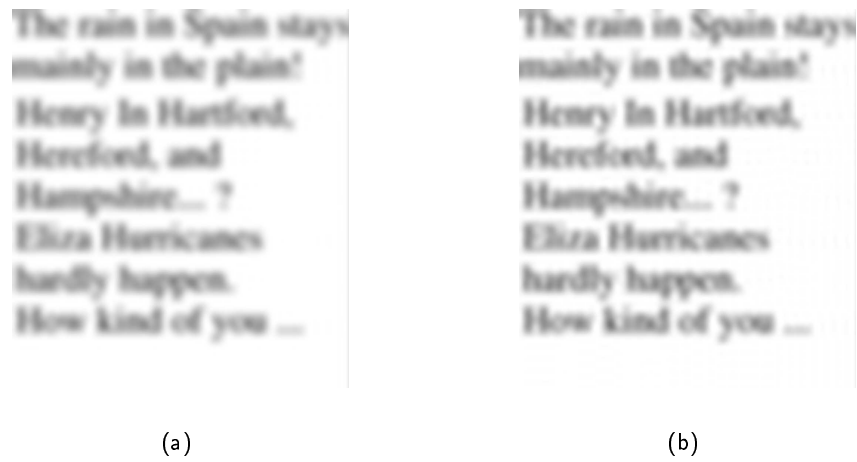
Figure 9.1: (a) prolate (b) SR filter. The text is more readable with the SR filter than with the prolate.
