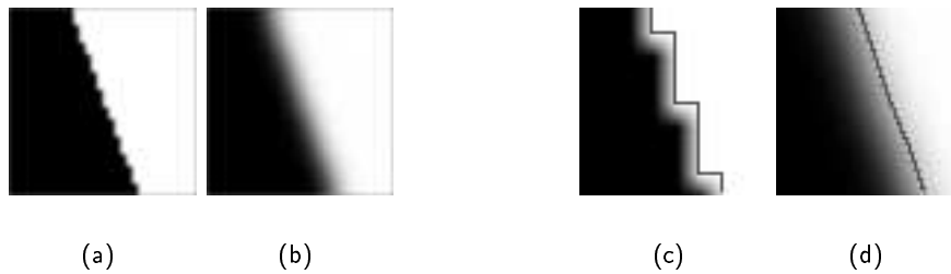
Figure 12.7: (a) Aliased image 128 \times 128 . (b) blurred image 128 \times 128 . (c) One level line on the zoomed version of (a). (d) One level line on the zoomed version of (b). Note the discontinuity and the regularity of the aliased and blurred image level lines, respectively.
