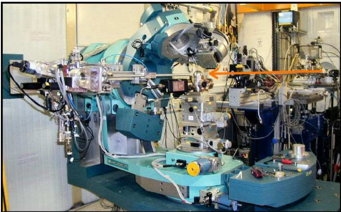
Figure 2.12: ID32 experimental hutch 1. Six-circle diffractometer. UHV baby chamber at the center of the diffractometer. The synchrotron beam is indicated by the arrow.
