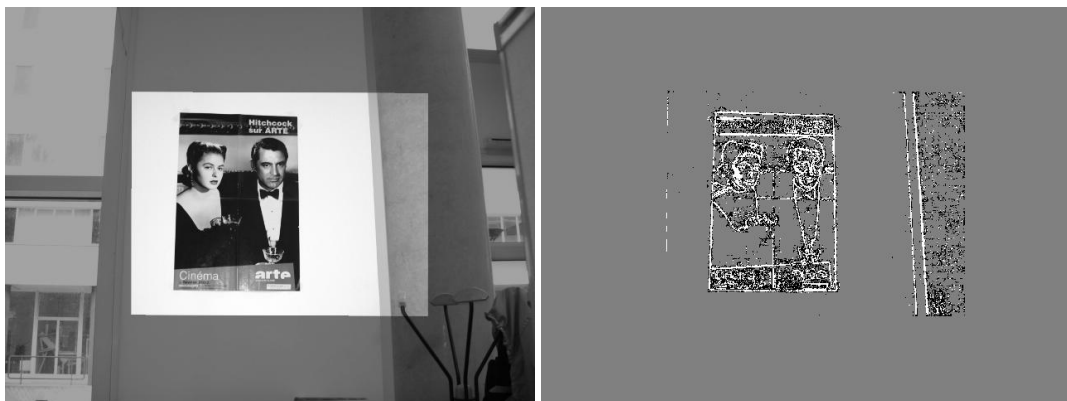
(b) Left: superimposition of the “scene image” and the transformed “target image”. Right: image of gradient orientation comparison.
