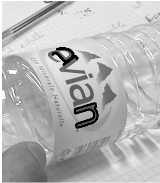
Figure 9.30: Evian: global similarity invariant matching. All 1-meaningful matches with character ‘n’ from the target image. The target ‘n’ is represented with 10 global shape elements, that match with 36 global shape elements from the scene image. The lowest NFA is 10^{-11} . False detections show NFAs between 0.7 and 1.
