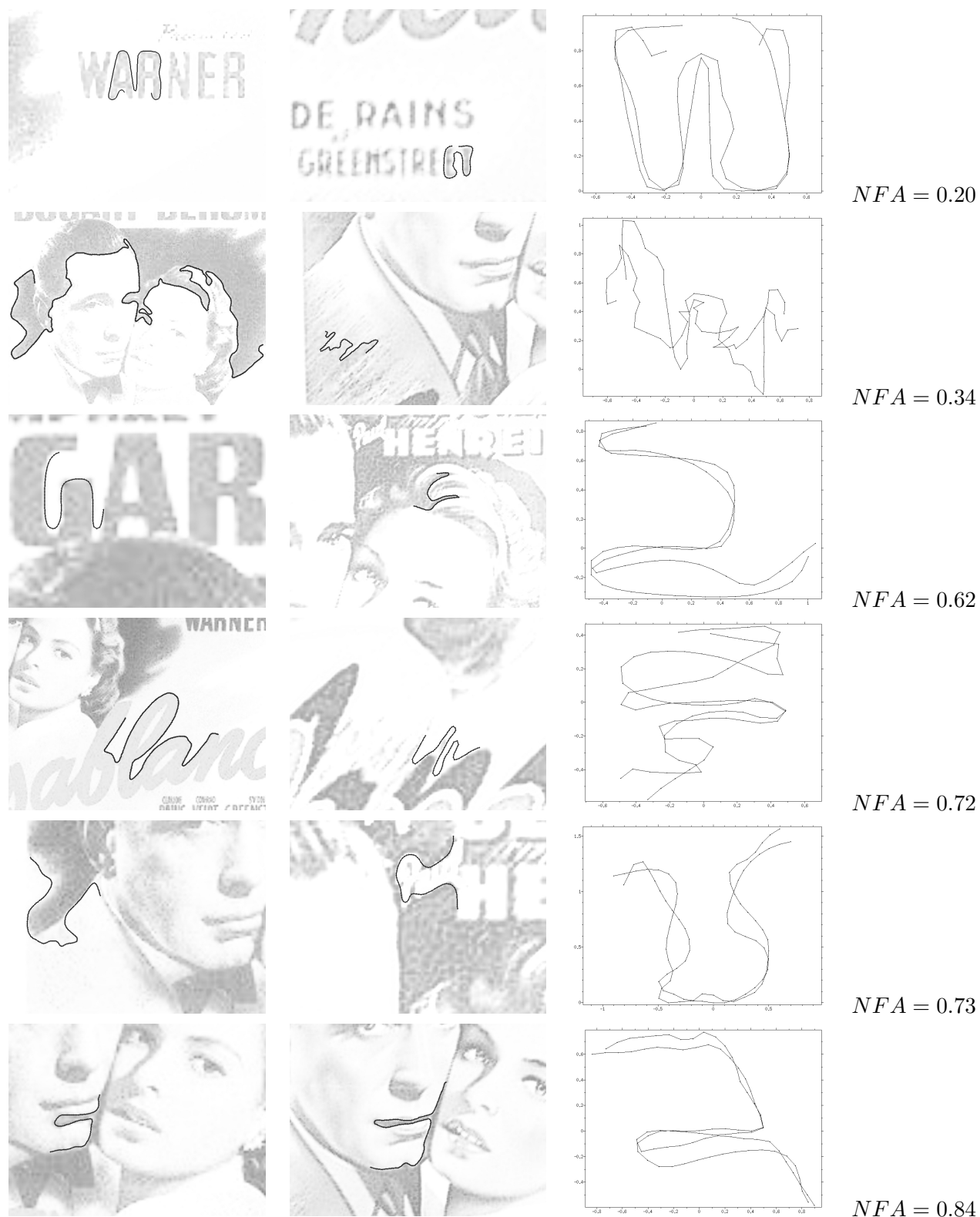
Figure 9.17: The six false matches for NFA < 1 , with their normalized codes. The left most and middle images correspond to the target and the scene shape elements, respectively. The right most image shows their normalized codes, superimposed. All false matches show NFA s between 0.1 and 1.
