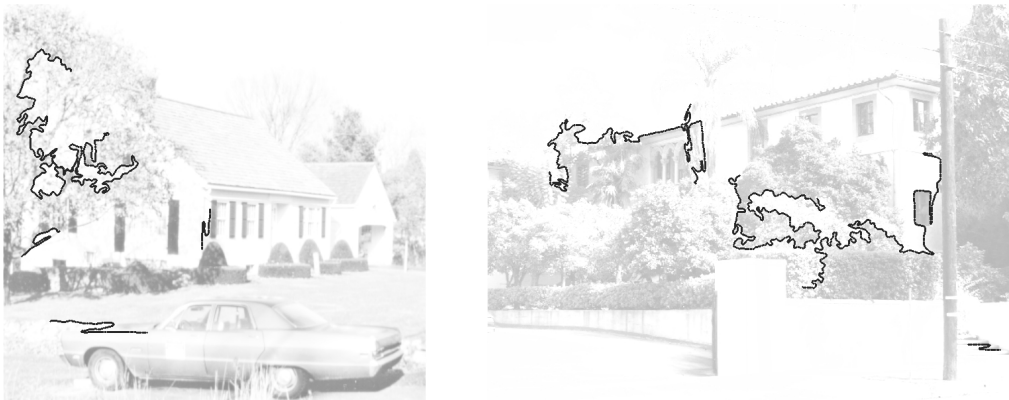
Figure 9.19: Left: target image; 4731 shape elements were extracted from this image. Right: scene image; the number of shape elements extracted from it was 4946. Among the 23 \cdot 10^6 pairs of target-scene shape elements, only six match at NFA < 1 . The NFA of these matches range from 0.21 to 0.97.
