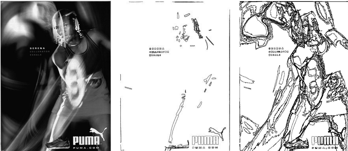
Figure 4.6: Influence of quantization noise on meaningful boundaries. On the left, the original image is coarsely quantized since it has a very low contrast. This leads to bad gradient estimation and a lot of missing detections (middle). Multiscale detection is less sensitive to quantization noise and leads to more correct detections (right).
