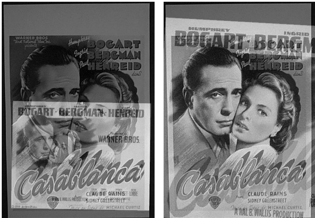
Figure 1.15: For each identified transform cluster, an “average” similarity transform is estimated. In order to check the consistency of the method, the target image is mapped over the database image, with each estimated transform. On the left, the average transform corresponding to the first maximal meaningful cluster maps both “Casablanca” word one on the other. On the right, the transform corresponding to the second maximal meaningful group maps the faces. Note the difference in scales.
