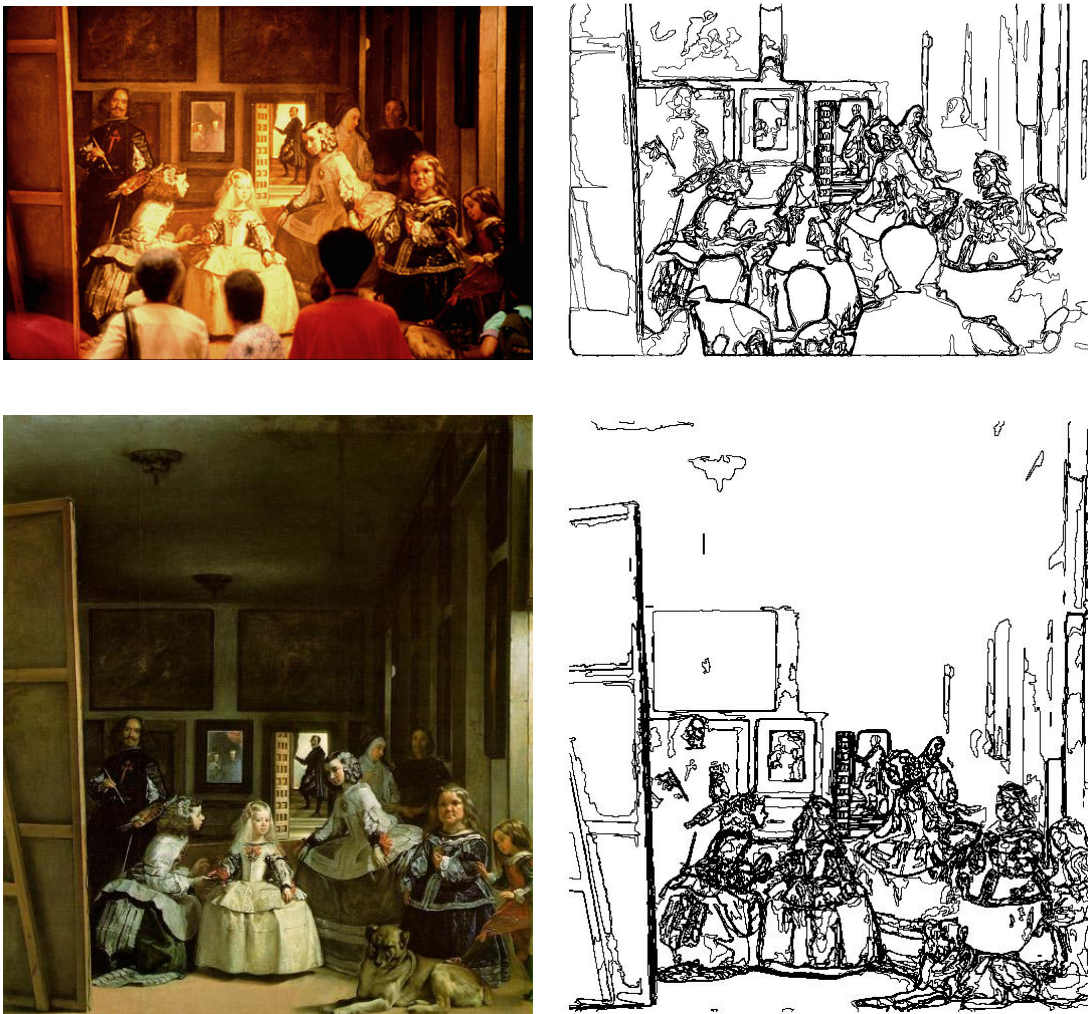
Figure 14.9: Las Meninas experiment. Top row: target image and its maximal meaningful boundaries. Bottom: scene image and maximal meaningful boundaries.
