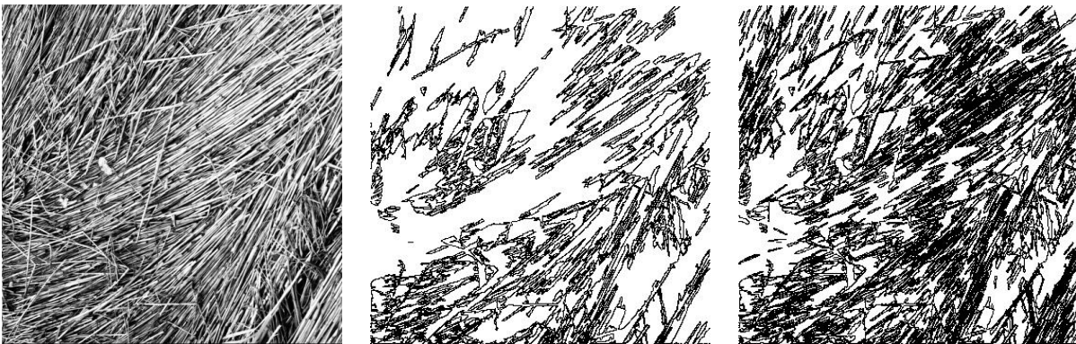
Figure 4.16: Influence of regularity. On the left, the original texture contains a lot of elongated structure. Because the texture shows large contrast variations, meaningfulness is a very strict criterion and contrasted meaningful boundaries miss many details (middle). In this case, local regularity is important and smooth and contrasted boundaries allow to retrieve missing lines.
