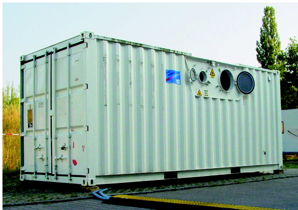
Figure 3.1: The "Teramobile" container next to the faculty of physics of the "Freie Universität Berlin". The small hole serves as the beam exit, while the big one is normally used for the telescope detection.
