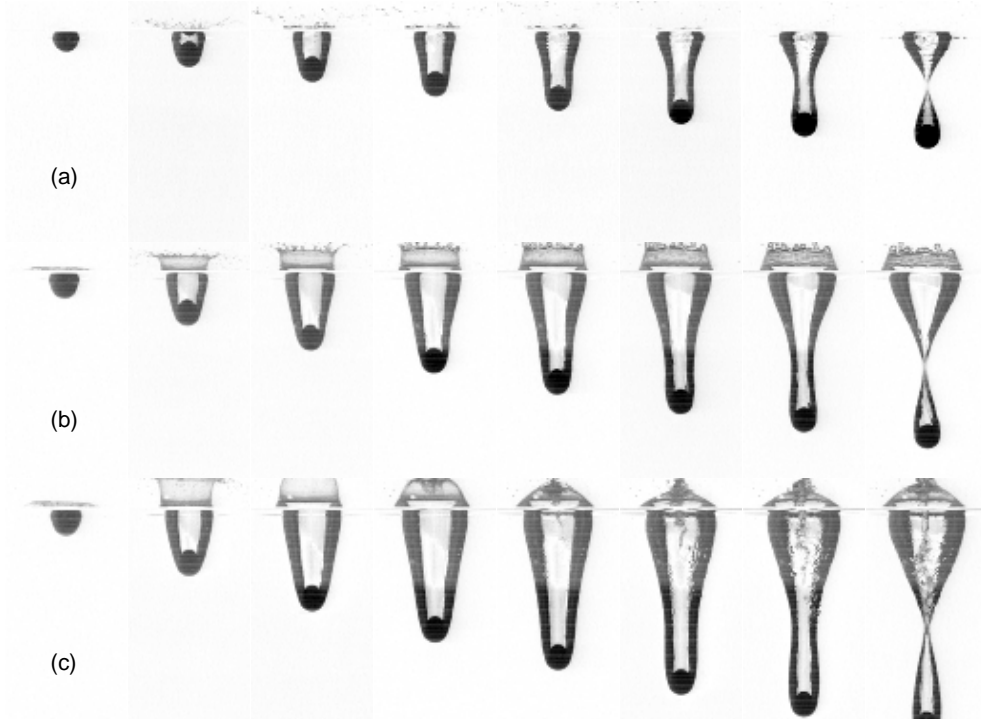
FIGURE 7. Influence of the impact velocity U for a fixed radius R_0 = 7.8 mm. The time step between the images is constant for the three chronophotographies \Delta t = 7.3 ms (a) U = 1.3 m/s, Fr = 22 (b) U = 2.4 m/s, Fr = 80 (c) U = 3.7 m/s, Fr = 188 .
