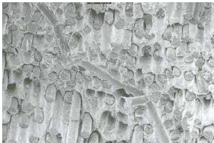
Figure 1: Misaligned fibres in a Ti/Al 2 O 3 system (R.R.Kieschke et. al , 1995).
