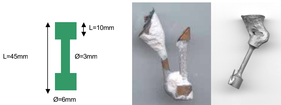
Figure 54: The centrifugal forces influence in the mould filling.
