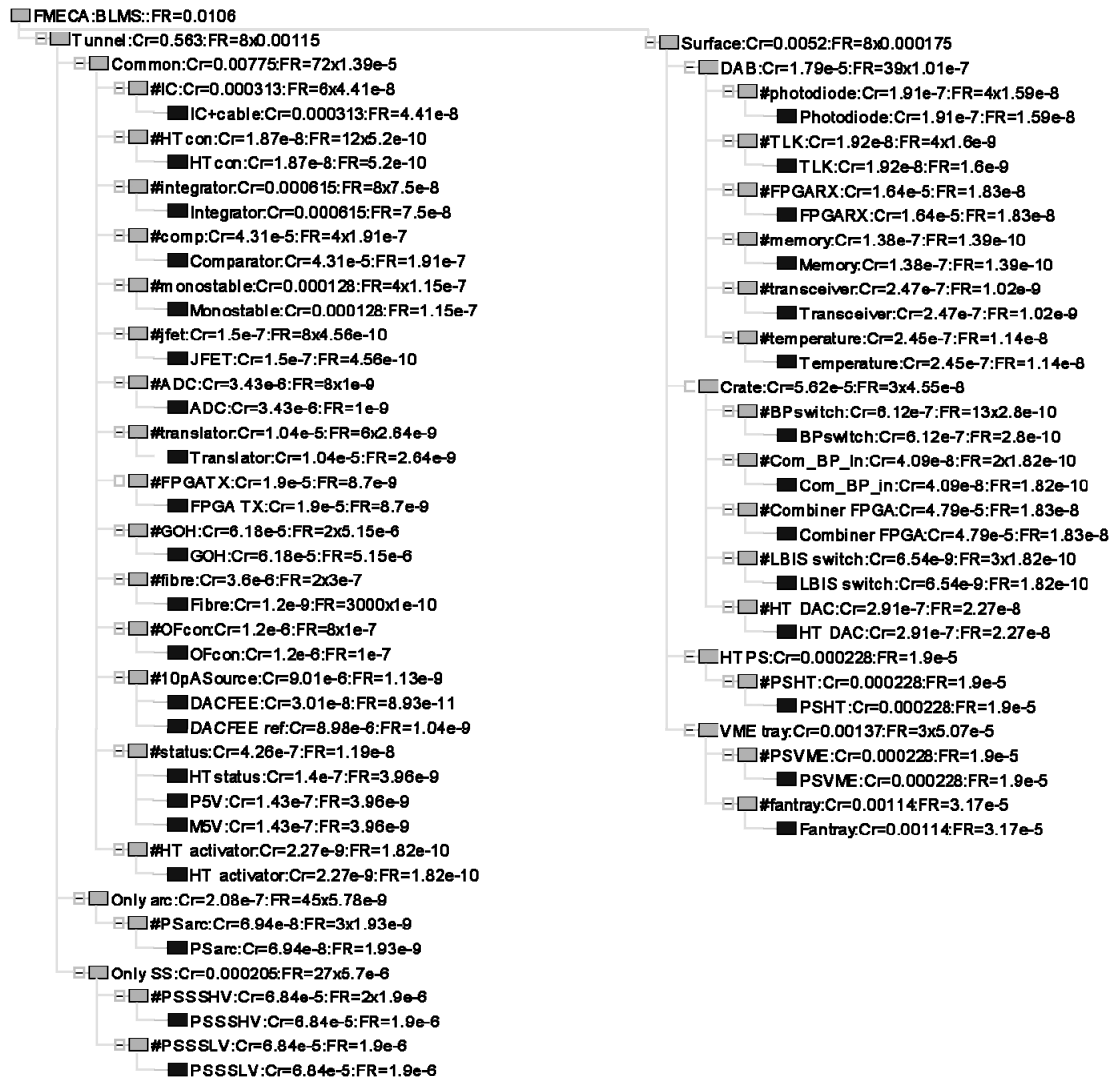
Figure B.5.1: Full diagram of the BLMS FMECA.
