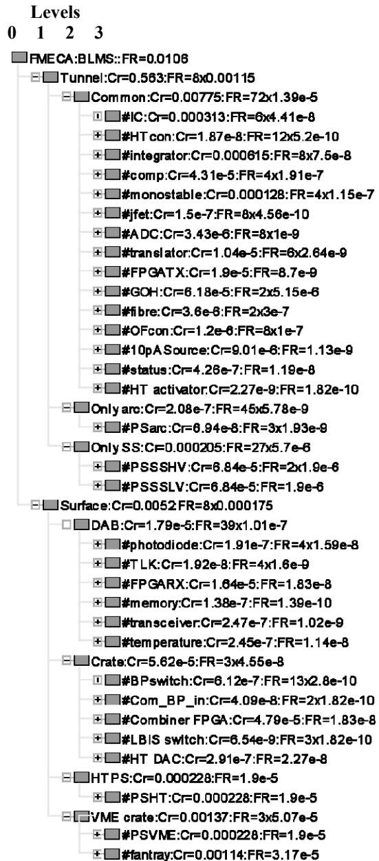
Figure 4.7: Diagram of the FMECA from level 0 to 3. Block name, criticalities and failure rates are reported.
