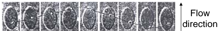
Figure 3.3: Top view of the tank-treading motion of a RBC highlighted by the movement of a bead attached to the membrane of the cell [58].
