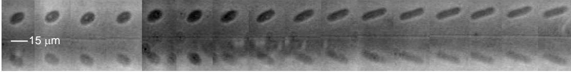
Figure 6.12: Sequence of deformation of a DMPC vesicle at \dot{\gamma}=2.7 \text{ s}^{-1} . The object tends to align with the flow direction as the ellipticity increases during the phase transition of the lipids. T between 18 and 27°C.
