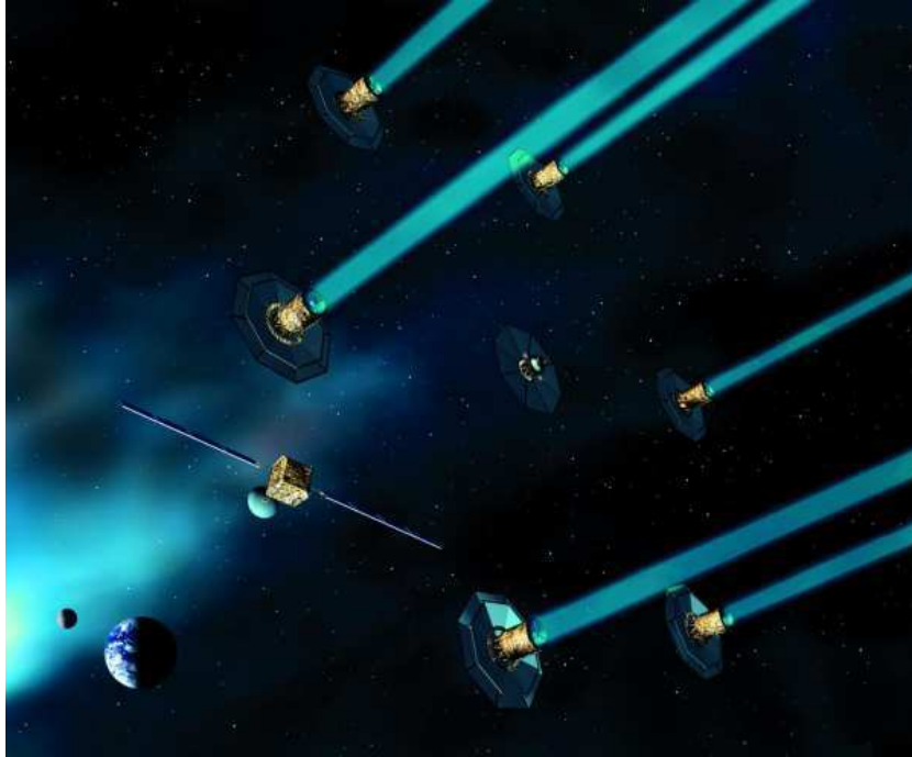
Figure 3: Artist impression of the Darwin space interferometer in its original hexagonal version, deployed and observing at the Sun-Earth Lagrange point L2. Added to the six telescopes are a central beam combining spacecraft and a satellite dedicated to communication and control (© 2002, ESA).
