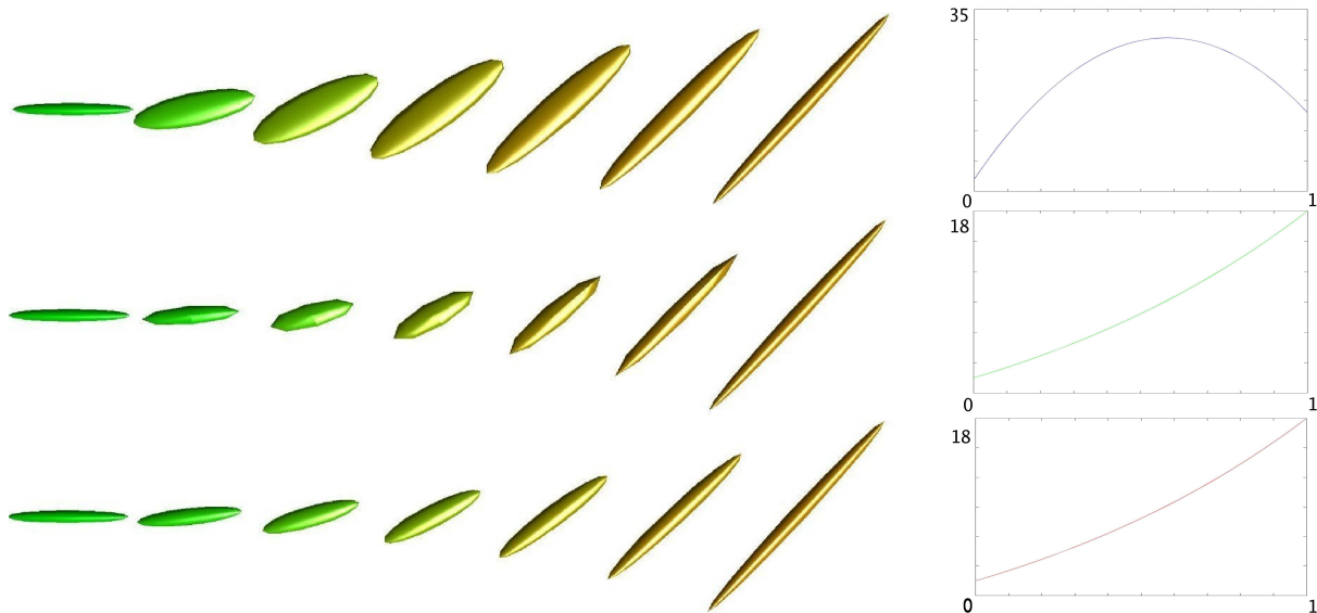
Figure 4.1: Geodesic interpolation of two tensors. Left: interpolated tensors. Right: graphs of the determinants of the interpolated tensors. Top: linear interpolation on coefficients. Middle: affine-invariant interpolation. Bottom: Log-Euclidean interpolation. The coloring of ellipsoids is based on the direction of dominant eigenvectors, and was only added to enhance the contrast of tensor images. Note the characteristic swelling effect observed in the Euclidean case due to a parabolic interpolation of determinants. This effect is not present in both Riemannian frameworks since determinants are monotonically interpolated. Note also that Log-Euclidean means are more anisotropic their affine-invariant counterparts.
