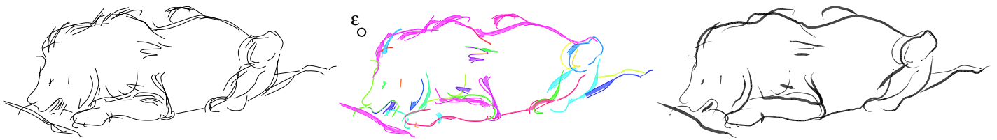
Figure 7.1: The two stages of our method. Lines of the initial drawing (left) are first automatically clustered into groups that can be merged at a scale \epsilon (each group is assigned a unique color). A new line is then generated for each group in an application-dependent style (at right, line thickness indicates the mean thickness of the underlying cluster).
