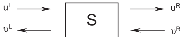
Figure 2.2: Scattering of plane waves. A right-moving arrow corresponds to the plane wave e^{ikx} , a left-moving arrow corresponds to the plane wave e^{-ikx} .
