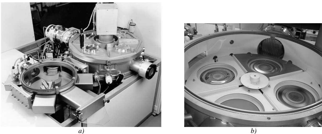
Figure 3.4 : a) Photograph of the DC-pulsed reactive magnetron sputtering equipment from Von Ardenne Anlagentechnik CS730S utilized in this work. At the front, the handler chamber with the glass top, at the back, the sputter process chamber. b) Photograph of the inside of the sputtering chamber showing 4 targets.
