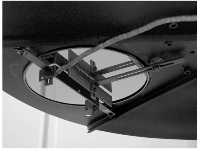
Figure 3.16 : Picture of the modified reactive magnetron sputtering system with additional electrodes positioned between target and substrate.
