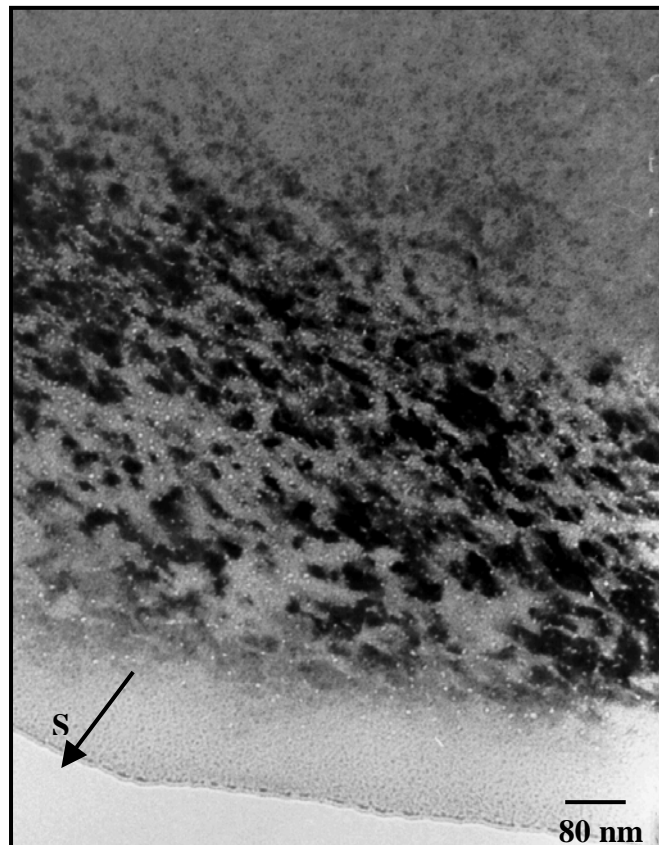
Figure 2.9: TEM image of helium implanted silicon at 50 keV and 5 \times 10^{16} \text{ cm}^{-2} , no anneal. See ref. [David et al. 2001]
