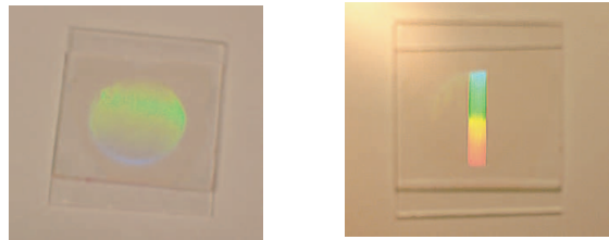
Figure 2.19 — Exemple de cellules H-PDLC.
