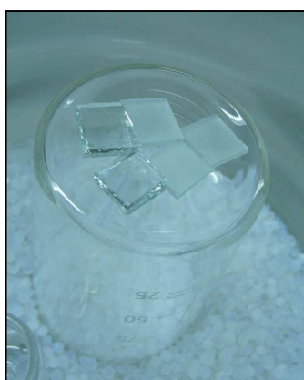
Figure V- 20: Photograph of the RG1 glass fragments appearance before (transparent squares) and after exposure to formic acid atmosphere (white squares) on the bottom of an upturned beaker.
