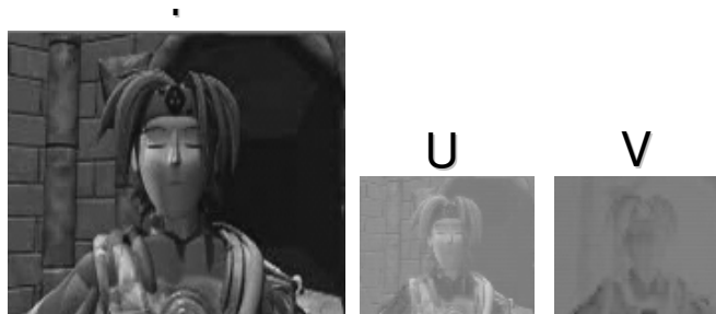
Figure 3. Color frame represented in YUV411 format
