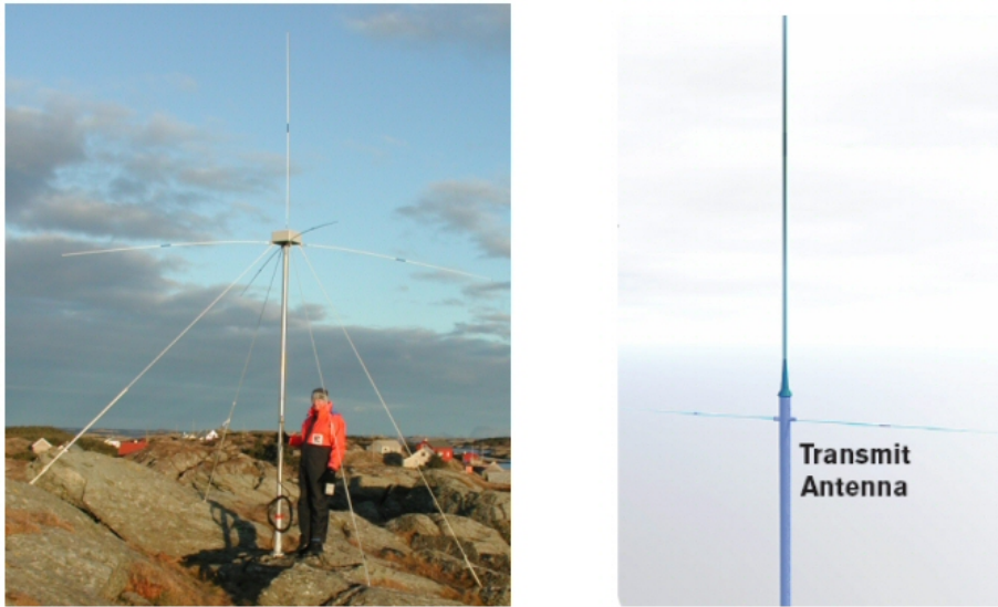
Figure 2.3: Example of antennas used in Sea Sonde system developed by CODAR Ocean Sensors. On the left, the receiving antenna and on the right the transmitting antenna
