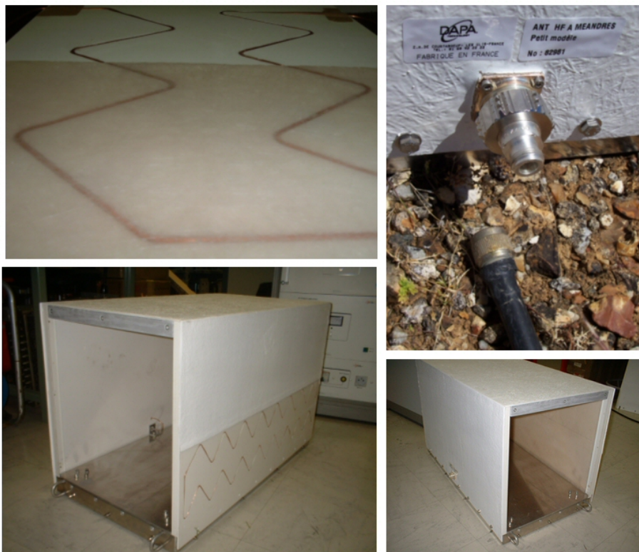
Figure 3.27: Pictures of the prototype and details of the final version of compact HF antenna
