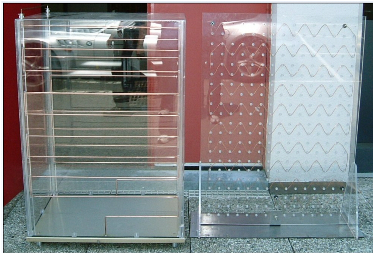
Figure 3.14: Comparison between double and sinusoidal MLA
