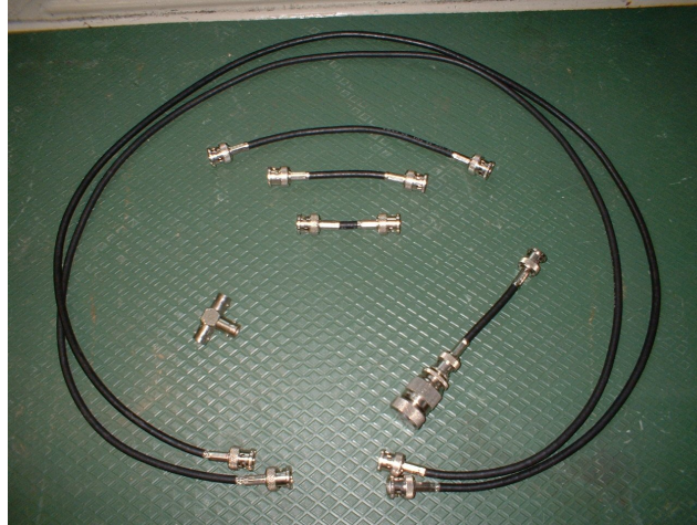
Figure 3.16: Stubs of different length prepared for matching experiment
