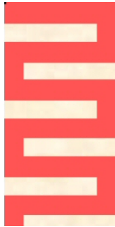
Figure 2.6: Example of a microstrip meander line antenna used for wireless communications
