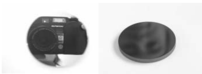
FIGURE 6 : Photos of a 10.1 micron thick EV-TAS1 film deposited on a As_2S_3 commercial target of 5 cm in diameter and further polished down to 0.2 micron.
