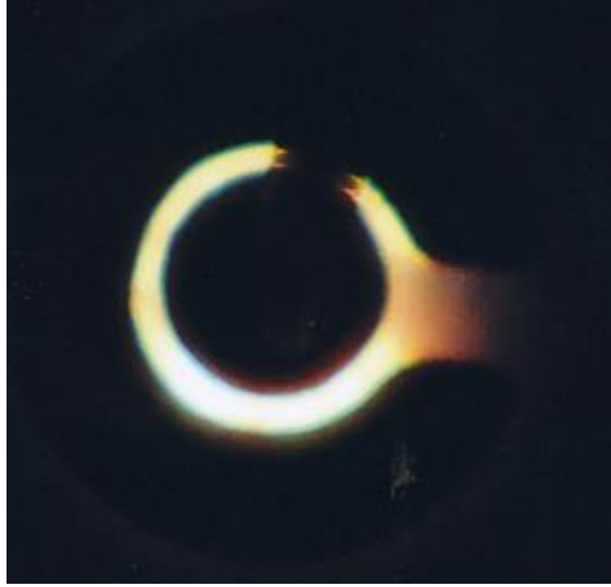
Figure 9.3: Photo of the EL from 5 stacks of GaN:Eu QDs capped with 10 nm Al_{0.5}Ga_{0.5}N:Si .
