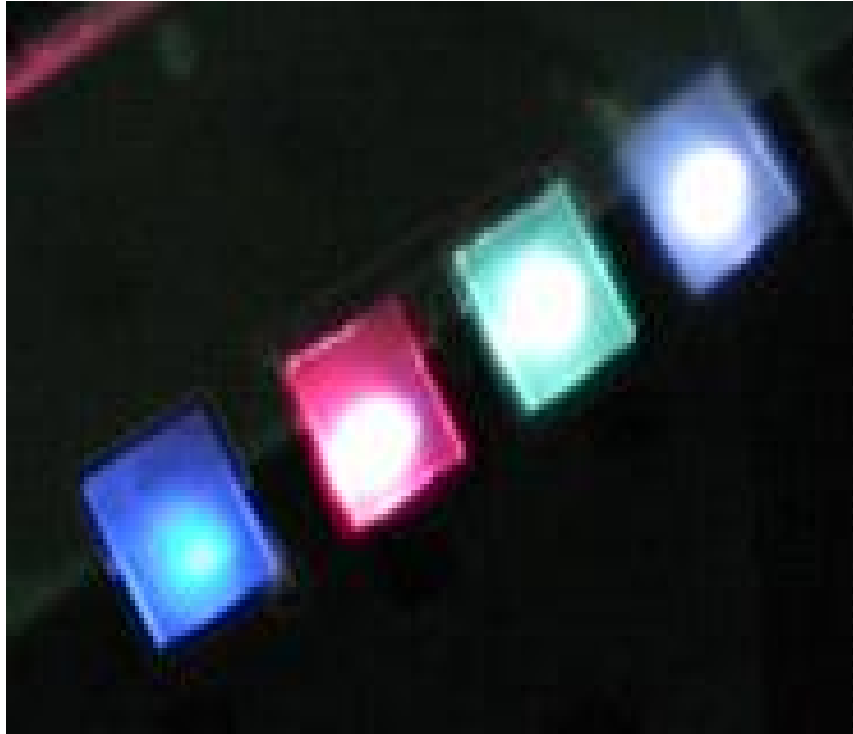
Figure 9.1: Photo of the PL of samples (from the left to the right) containing 100 stacks of GaN:Tm QDs, 100 stacks of GaN:Eu QDs, 100 stacks of GaN:Tb QDs and 24 x (4 stacks of GaN:Tm QDs, 6 stacks of GaN:Tb QDs and 2 stacks of GaN:Eu QDs).
