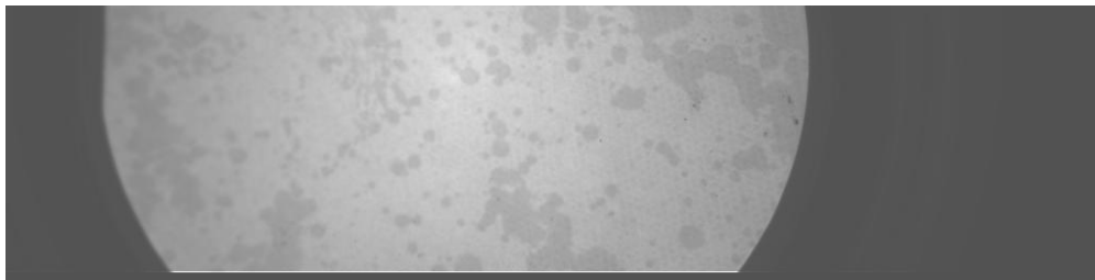
Figure 4-16: Flat field obtained with the DELFT image intensifier: the illuminated area is limited due to an inadequate optical coupling.
